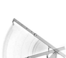
Hydraulic inclination of the jib
